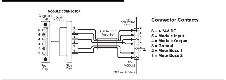
Fig. 23 - Module Connector Contacts Diagram
